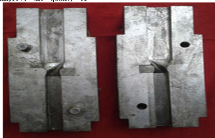
Fig. 1. The two parts of the TE mold [10].
